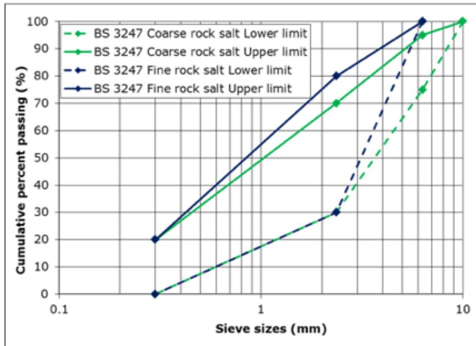
Figure 3.8.1 – BS3247 Upper and lower limit for grading of fine & coarse UK rock salt
