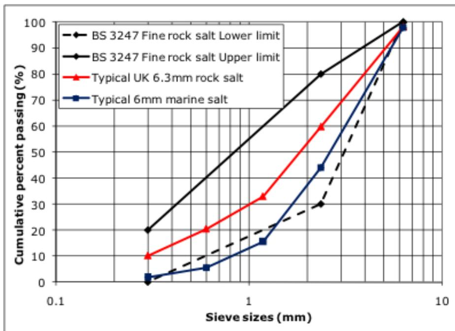
Figure 3.8.2 – Typical & BS3247 limits to gradings for fine & 6.3mm UK rock salt & 6mm marine salt
