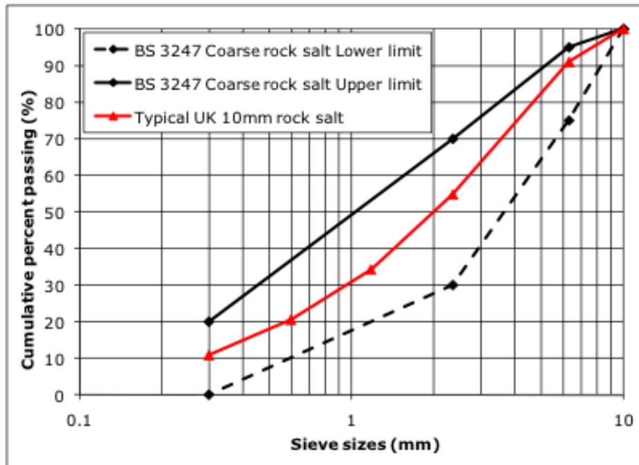
Figure 3.8.3 - Typical & BS3247 limits to grading for 10mm UK rock salt
