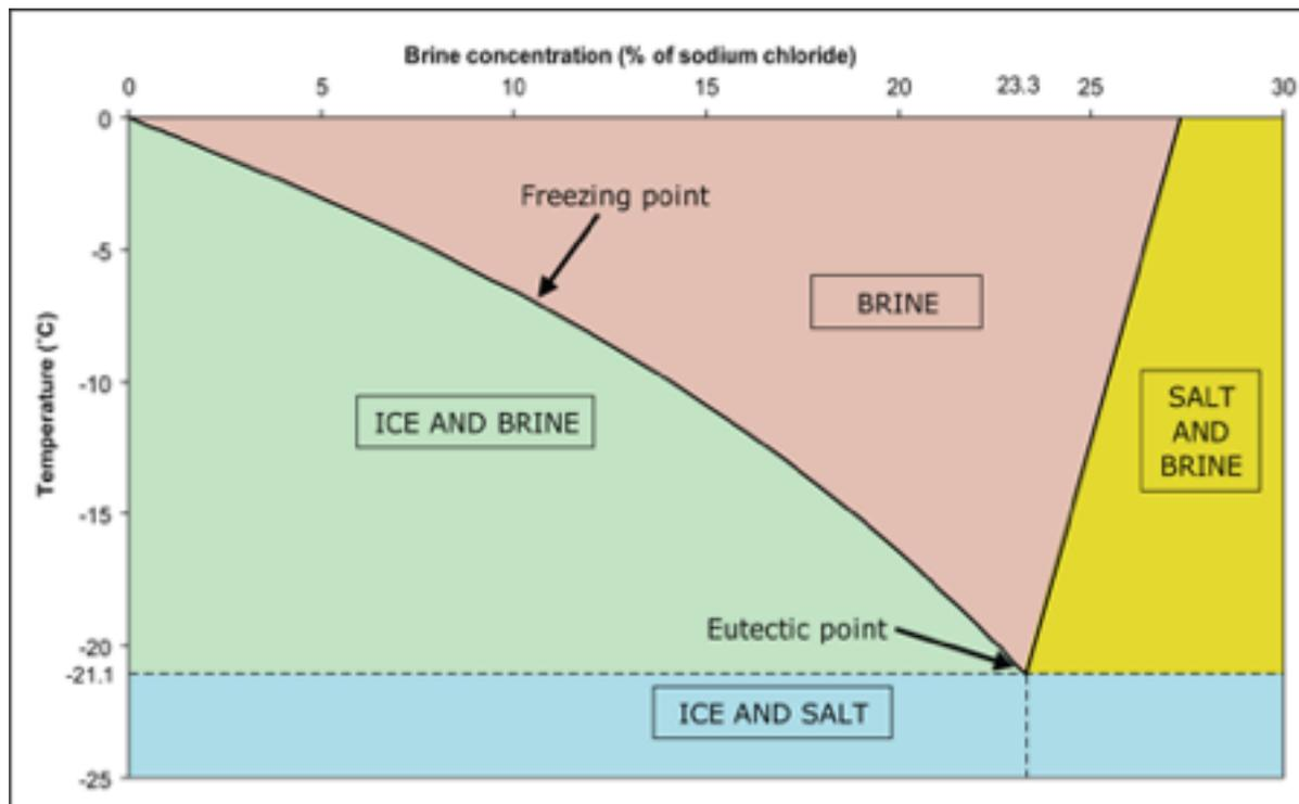
**Figure 3.6.1 - Phase diagram for sodium chloride and water**
