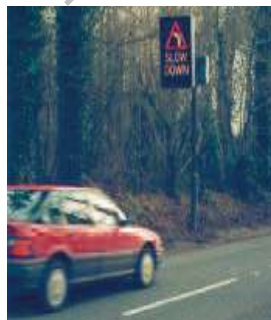
Vehicle Activated Sign (VAS) on approaches
